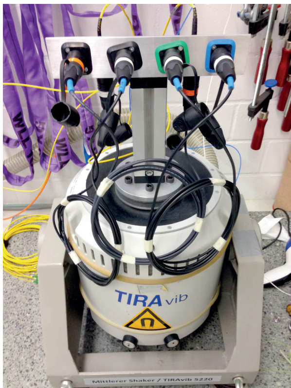
figure 2.a: : Vibration equipment and test cable arrangement
